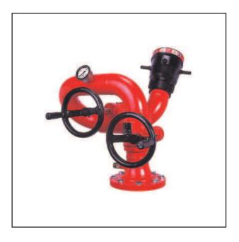
and epoxy painted for excellent corrosion resistance. The vertical and horizontal rotation is through corrosion resistant bronze swiveling joints with double row of stainless steel ball bearing. Both vertical and horizontal movement are controlled with handwheel driven fully enclosed worm gears and protect from the elements.
